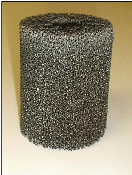
Figure 4.1: Ceramic body of the porous burner
