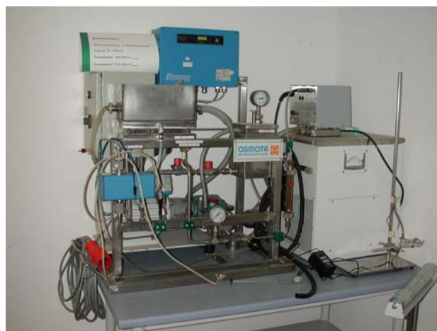
Figure 3: Experimental plant of membrane distillation
